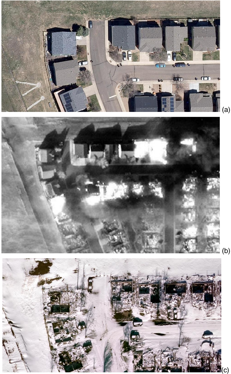
Figure 2-5. Examples of satellite imagery to evaluate spatial features: (a) before, (b) during (2 PM MST), and (c) after (2 Jan. 2022, vexcel 7.4 cm) in Sagamore Neighborhood (39°57'25.7" N, 105°10'41.5" W)
